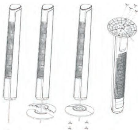
The stand (4 and 5) for the upright comes in two parts which can be very easily fitted around the base of the appliance. One part of the stand (4) should be placed on the front of the appliance base and the second section of the stand (5) - the one with the opening on the outside for the electrical cable (6) - should be placed at the back.
