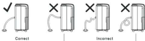
**Note:** If you do not require the continuous emptying function, remove the drainage tube (10) and correctly replace the tank chip (9) and then the tank (3).
